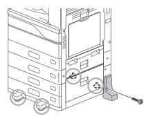
Before moving the equipment with the Desk installed, remove the front stabilizer. Be sure to reinstall it after the equipment has been moved.
