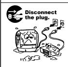
If foreign objects (metal fragments, water, liquids) enter the machine, turn off the power switch and disconnect the power cord plug from the outlet, and then contact your authorised Toshiba Tec Corporation representative for assistance. Continued use of the machine in that condition may cause **fire** or **electric shock**.
