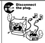
Continued use of the machine in an abnormal condition such as when the machine is producing smoke or strange smells may cause fire or electric shock. In these cases, immediately turn off the power switches and disconnect the power cord plug from the outlet. Then, contact your authorised Toshiba Tec Corporation representative for assistance.
