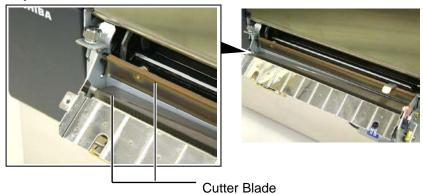
**5.** Reassemble in the reverse order of removal. Secure the Media Guide by the hook.
