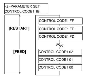
After setting the control code for Control Code 1, press the **[PAUSE]** key to show the CONTROL CODE2 screen. In a same manner, press the **[PAUSE]** key after setting the control code for Control Code 2 to display the CONTROL CODE3 screen.
