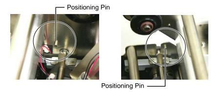
(2) Fit the tip of the Pinch Roller Plates into the slot in the Ribbon End Sensor.
