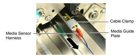
**9.** Remove jammed media from the media path. DO NOT USE any sharp implements or tools as these could damage the printer
