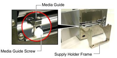
10. Place the assembled Media Holder onto the Supply Holder Frame, and feed the media between the two Media Guides.
