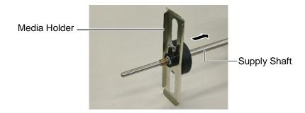
2. Turn the Locking Lever of the Media Holder to "Close" position to fix the Supply Shaft with the Media Holder.
