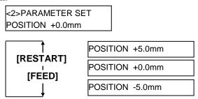
**[FEED]** key: Pressing the **[FEED]** key one time causes a -0.1mm change,
