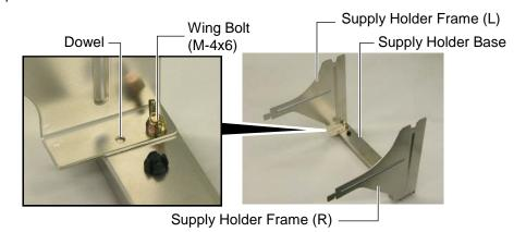
**2.** Attach the assembled Supply Holder Frame to the rear of the printer by inserting the hooks of the Frame into the two slots in the rear of the printer, as shown below.
