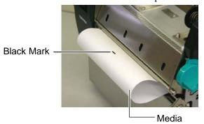
(2) Move the Movable Sensor by rotating the Adjustment Knob, until the Black Mark Sensor aligns with a black mark. (The left side hole indicates the position of the Black Mark Sensor).
