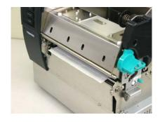
**12.** Move the Media Guides inside, causing the media to be automatically centred. Then, tighten the Media Guide Screws to secure the Media Guides.
