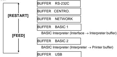
After selecting the receive buffer, press the [PAUSE] key.
