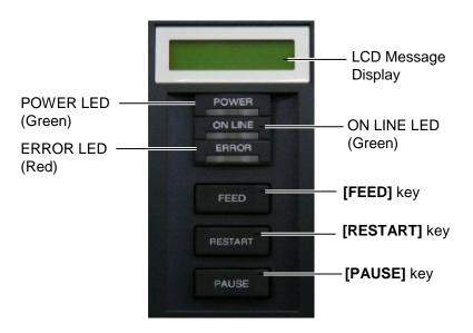
The LCD Message Display shows messages in alphanumeric characters and symbols to indicate the printer's current status. Up to 32 characters can be displayed on two lines.
