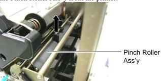
**10.** Wipe the Pinch Roller Ass'y with a soft cloth slightly moistened with absolute ethyl alcohol.
