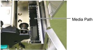
10. Wipe dust and adhesive off the Media Guides with a soft cloth moistened with alcohol.
