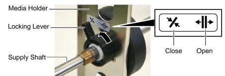
**3.** Place a media roll onto the Supply Shaft and push the media against the Media Holder.
