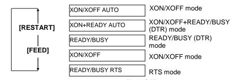
After selecting a flow control code, press the **[PAUSE]** key.
