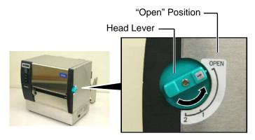
**2.** Open the Top Cover, Right Side Cover, and the Head Lock Plate.
