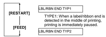
TYPE2: When a label/ribbon end is detected in the middle of printing, the printer prints the half-finished label as far as possible, and stops when the next label is at the home position.
