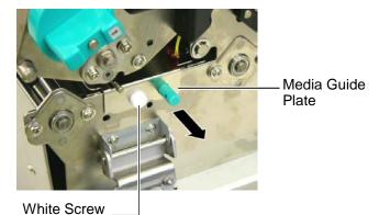
**6.** When the Media Guide Plate is slightly pulled, the first Cable Clamp can be seen. Release the Media Sensor Harness from the Cable
