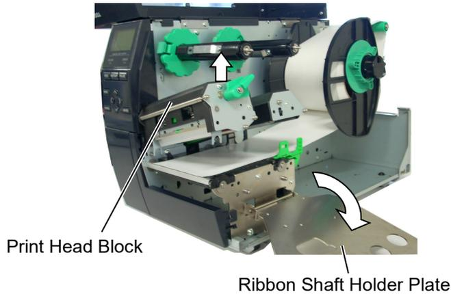
5. Remove the jammed media from the printer. DO NOT use any sharp implements or tools as these could damage the printer.
