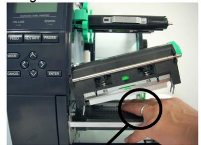
Care must be taken not to allow a metal object like a ring to touch the print head edge.
